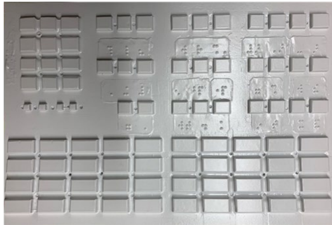
Figure 7 Model of a keyboard made with thermoforming
