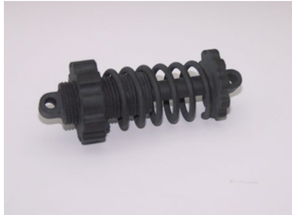
Figure 5 Freedom of shape. Both models were printed in one process
